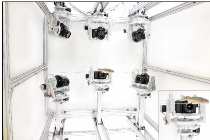
Figure 1. Working prototype of 6 camera COPIS installation showing specimen mounted on two strands of monofilament in specimen staging area.
