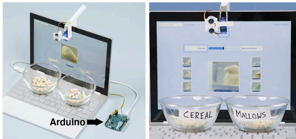
Figure 2: A tiny sorter project made of Arduino, cardboard, googly eyes, and the Google AI education platform. The tiny sorter categorizes whether an item is a marshmallow or a piece of cereal (Google, 2020b). For this project, students first collect images of pieces of cereal and marshmallows to train an AI system. Then, they develop paper structures with googly eyes that can physically sort cereal and marshmallow and connect them to an Arduino, a microcontroller (an easy-to-use open-source electronic prototyping platform).
