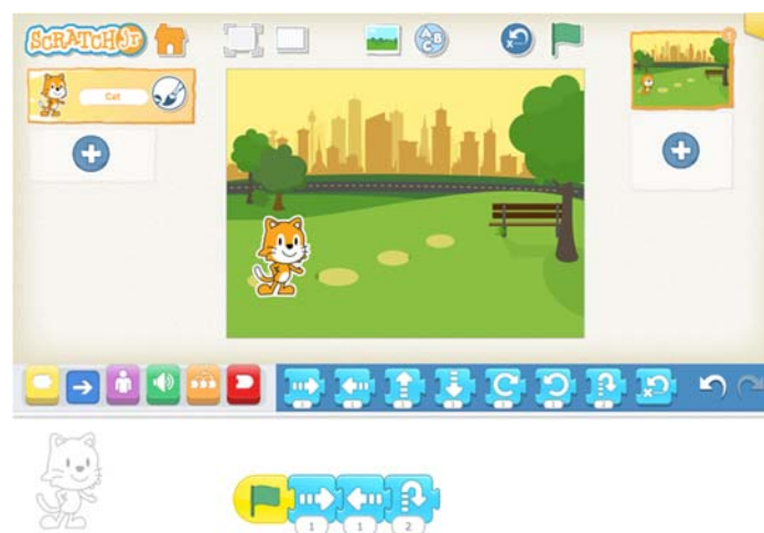
Figure 1 ScratchJr interface. Puzzle-piece shaped blocks with iconic images represent different actions that characters, or sprites, can take on the screen.
